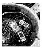
III. Secure the inner black lid to the dry shipper using the (1) corresponding hole through both the dry shipper and inner black plastic lid with the supplied zip tie.
